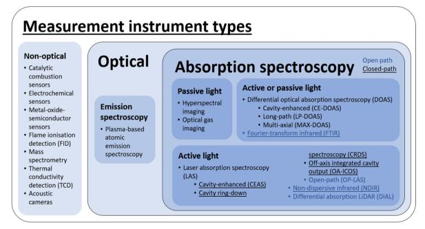
Fig. 7 Taxonomy for describing and categorising measurement instruments with example techniques. The techniques listed are not exhaustive. Keywords are defined in the lexicon in the ESI.† Optical absorption spectroscopy instruments which typically make use of open-path light sources are highlighted in blue. Optical absorption spectroscopy instruments which typically make use of closed-path light sources are underlined.
