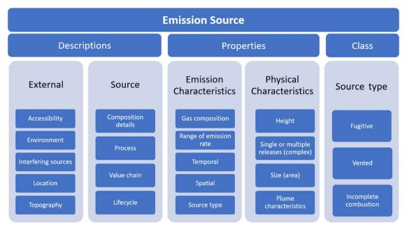
Fig. 4 Taxonomy for describing and classifying emission source properties and characteristics. Many of the emission source properties could benefit from additional description or context (for example, preferred units of measurement). Keywords are defined in the lexicon in the ESI.†
