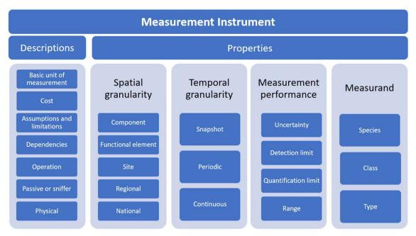
Fig. 6 Taxonomy for describing and classifying a method element (in this case, the measurement instrument) and its properties. Keywords are defined in the lexicon in the ESL:†
