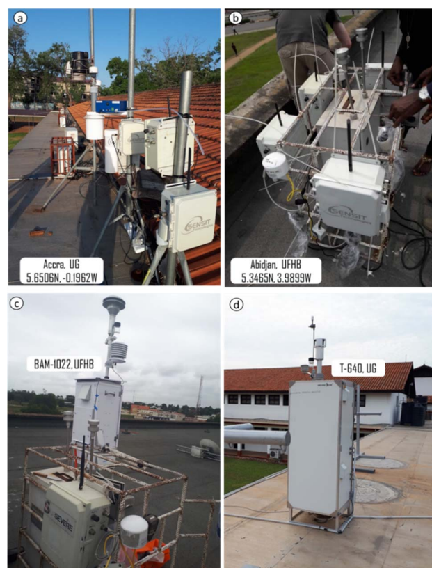
Fig. 2 Pictures of monitors, (a) RAMPs at UFHB, (b) RAMPs at UG, (c) collocation of BAM-1022 and RAMPs at UFHB, (d) Teledyne T-640 at UG.
