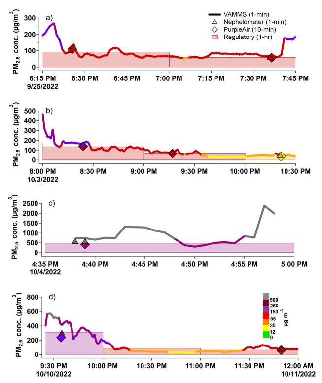
Fig. 1 Timeseries of VAMMS (1 min), nephelometer (1 min), PurpleAir (10 min), and BAM 1022 (60 min) PM<sub>2.5</sub> measurements at the Oakridge, OR air quality monitoring station during the Cedar Creek fire for four sampling days (a–d), colored by the corresponding "approximate AQI" category. Data from the nephelometer and PurpleAir are shown only when the VAMMS was within 400 m of them. The timestamp is given in universal coordinated time.
