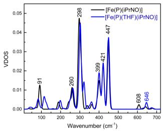
Fig. 7 Top panel: NRVS-derived vibrational density of states (VDOS) for [ $^{57}$ Fe(TPP)(THF)(iPrNO)] (black) and the  $^{15}$ N-labeled iPrNO complex (blue). Bottom panel: BP86/TZVP calculated NRVS VDOS for [Fe(P) (iPrNO)] (black;  $P^{2-}$  = porphine dianion) and [Fe(P)(THF)(iPrNO)] (blue).
