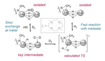
Fig. 3 Demonstration of the reactivity of metalated ligands in the activation of H<sub>2</sub>. Deuteration studies show metal based H/D exchange is slow with the tetrahydrido dimer while the metalated trihydrido complex reacts with  $H_2/D_2$  quickly. L =  $Me_4$ -TACD.†
