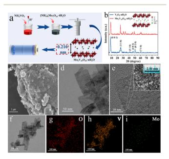
Fig. 7 (a) Schematic of the sample preparation of  $Mo_3V_{15}O_{35}\cdot nH_2O$ . (b) XRD patterns of  $V_2O_5\cdot nH_2O$  and  $Mo_3V_{15}O_{35}\cdot nH_2O$ . (c) SEM image, d and (e) TEM and HRTEM images, and (f–i) TEM elemental mapping images of  $Mo_3V_{15}O_{35}\cdot nH_2O$ . Reproduced with permission from ref. 148. Copyright (2024), Elsevier.
