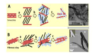
Fig. 2 Synthesis of smectites (A) of fibrous clays and (B) semiconductor nanoarchitectures *via* the three-step "organoclay colloidal route": (a) formation of an organoclay due to the replacement of the interlayer cations by alkylammonium ions, (b) treatment with metal oxide precursors and (c) calcination to obtain nanoarchitectures containing the semiconductor, reproduced with permission from ref. 24. Copyright 2019. Beilstein-Institut.
