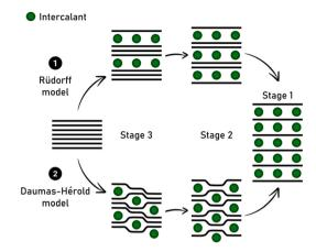
Fig. 4 Schematic representation of the Rüdorff model versus the Daumas-Hérold model, considering the flexible feature of graphene sheets. This model describes the continuous transformation from third to second stage GIC.
