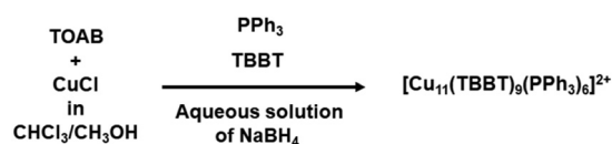
Fig. 6 Synthesis procedure of [\text{Cu}_{11}(\text{TBBT})_9(\text{PPh}_3)_6]^{2+} NC.
