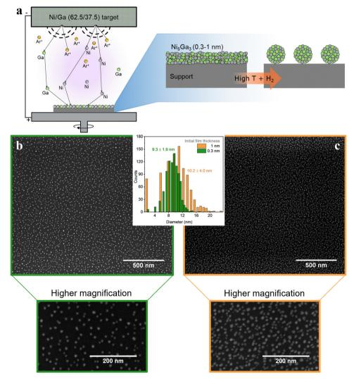
Fig. 8 (a) Nanoparticle synthesis schematics, combining magnetron sputtering and annealing; (b) and (c) Ni<sub>5</sub>Ga<sub>3</sub> thin films of 0.3 (green) and 1 nm (orange), respectively, on an SiO<sub>2</sub> (50 nm)/Si (350 μm) support annealed at 750 °C for 30 min in 10% H<sub>2</sub> in He. SEM images were acquired at 5 kV and 0.1 nA.
