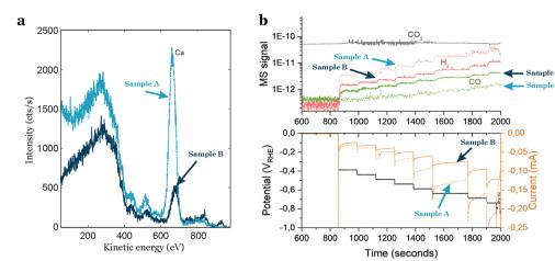
Fig. 4 Impact of impurities in the support on the electrocatalytic activity of a sample. (a) ISS spectra of two glassy carbon supports from the same batch, but with different amounts of impurities. (b) Electrochemical performance of 3.5 nm Au nanoparticles with 5% coverage of the electrode. The sample contaminated by the support exhibits increased H<sub>2</sub> production, overshadowing the CO<sub>2</sub>R activity
