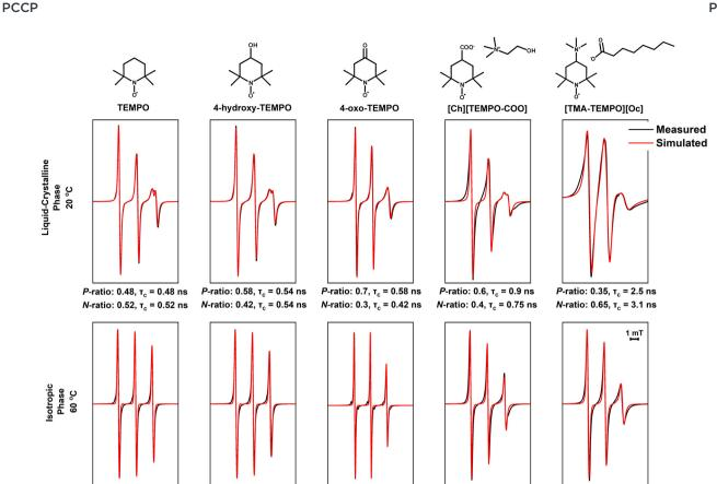
Fig. 10 Measured (black) and simulated (red) X-band CW EPR spectra of 1 mM of the studied spin probes in CAOC. The measurements were performed at 100 kHz mod. frequency and 1 mW microwave power. *P* is the population of the polar domain and *N* the population of the non-polar domain. These same simulation values (see ESI,† Table S5) were used in fitting each set of spectra; the isotropic phase was simulated using only the non-polar population parameters.
