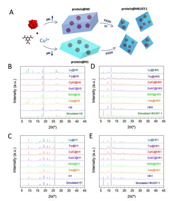
Fig. 4 (A) Schematic representation of the protein@HKUST-1 synthetic procedure. XRPD patterns of the (B) protein@H0, (C) protein@H1, (D) protein@HKO and (E) protein@HK1 biocomposites.
