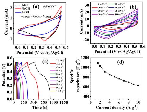
Fig. 3 (a) Comparative CV curve for different electrolytes, (b) CV at various scan rates, (c) GCD at different current densities, and (d) specific capacitance vs. current density for Co-CP in 7 M NaOH.
