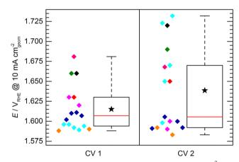
Fig. 6 Comparison of KPI of the standard electrode at  $10 \text{ mA cm}^{-2}$  before (CV 1) and after (CV 2) the stability measurement. The color code corresponds to the color code used in the previous figures. For CV 1 only the data points of electrodes are shown that endured the stability measurement
