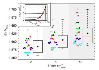
Fig. 4 Key performance indicators for 2, 5, and 10 mA cm $^{-2}$  deduced from "CV 1" (as shown on an exemplary curve in the inset) measured on the standard catalyst by 11 different laboratories/experimenters. In all cases, the standard protocol was followed for both, sample preparation and experiment execution. Different colors indicate different laboratories/experimenters; the box plot format is explained in detail in the text.
