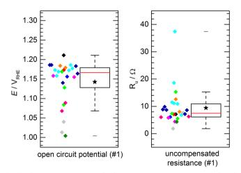
Fig. 3 Open circuit potentials (left) and uncompensated resistance (right) of the activated standard electrodes (100  $\mu g$  cm $^{-2}$  nickel–cobalt–oxide nanopowder). Measurements were performed by 11 different laboratories/experimenters, indicated by different colors. The box plot representation is explained in the text.
