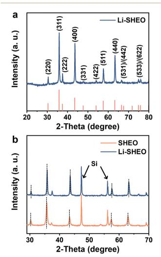
Fig. 1 XRD patterns of (a) Li-SHEO material, and (b) SHEO and Li-SHEO materials for revealing the peak shift behaviour.
