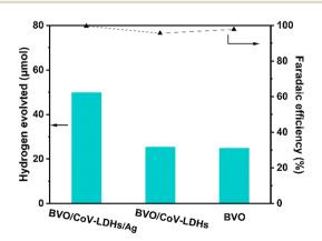
Fig. 5 Measured hydrogen gas and the Faradaic efficiencies of hydrogen evolution on various photoanodes at 1.2 V under AM 1.5 G illumination; the electrolyte was 0.5 M  $\rm Na_2SO_4$  solution with 0.1 M glycerol.
