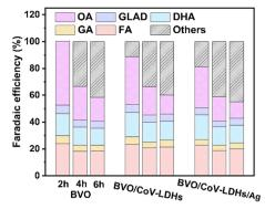
Fig. 4 The Faradaic efficiencies toward various oxidation products in 0.5 M  $Na_2SO_4$  solution with the presence of 0.1 M glycerol at 0.8 V vs. RHE, and the gray area depicts the oxidation products not in the solution, likely  $CO_2$ .
