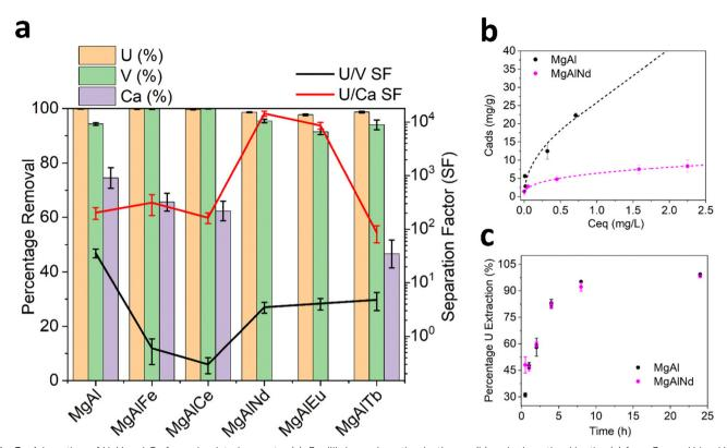
Fig. 3 Adsorption of U, V and Ca from simulated seawater (a). Equilibrium adsorption isotherms (b) and adsorption kinetics (c) from 3 ppm U in pH 8  $Na_2CO_3$ . Markers = experimental data, lines = fitted Freundlich isotherm model.
