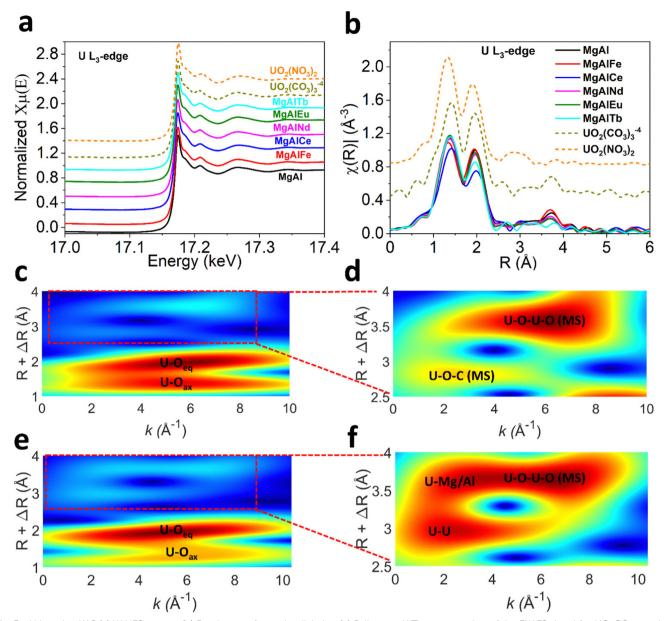
Fig. 5 U L<sub>x</sub>-edge XAS (a) XANES spectra (b) Fourier transformed radial plot. (c) Full-range WT representation of the EXAFS signal for UO<sub>2</sub>CO<sub>x</sub> standard (1-4 Å) and  $k_2 = 0-10$  (d) Magnified high-R WT region for UO<sub>2</sub>CO<sub>3</sub> standard (2.5-4 Å and  $k_2 = 0-10$ ) (e) full-range WT for MgAl (1-4 Å and  $k_2 = 0-10$ ) (f) Magnified high-R WT region for MgAl (2.5–4 Å and  $k_2 = 0-10$ ).
