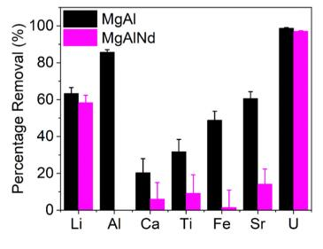
Composition of spiked seawater and adsorption of trace elements from spiked seawater with MgAl and MgAlNd LDH samples
