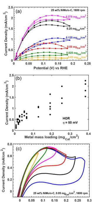
**Fig. 6** Evidence for mass transfer limitations and oxidative catalyst deactivation. (a) Representative steady-state voltammograms for the HOR on Ni–Mo/oC over a range of catalyst mass loadings. (b) Full dataset compiling HOR current density as a function of mass loading. (c) Representative cyclic voltammetry data collected at a scan rate of 0.5 mV s $^{-1}$  over a range of positive potential limits.
