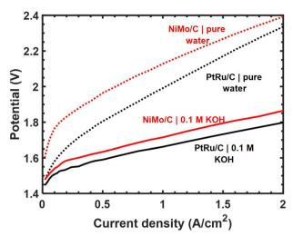
Fig. 4 Polarization data for full HEM electrolysis using 25 wt% Ni–Mo/o-C and Pt–Ru/C (50 wt% Pt, 25 wt% Ru) cathodes using aryl-ammonium based membrane/binder polymers and IrO $_x$  anode catalysts. The total catalyst loading of Ni–Mo/oC was 1 mg $_{\rm cat}$  cm $^{-2}$  and for Pt–Ru/C it was 0.15 mg $_{\rm cat}$  cm $^{-2}$ . Unsupported IrO $_x$  nanoparticle anodes were loaded at 3 mg $_{\rm cat}$  cm $^{-2}$ .
