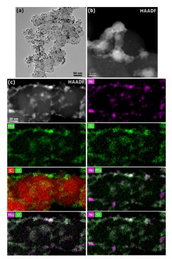
Fig. 2 TEM and HAADF-STEM image of 25 wt% Ni-Mo/o-C. (a) Bright field image depicting a representative nanoparticle/carbon composite; (b) HAADF dark field image depicting a nanoparticle agglomerate on the carbon support; (c) multipanel overlay of HAADF image and EDS maps demonstrating the spatial distribution of Ni, Mo, and O.
