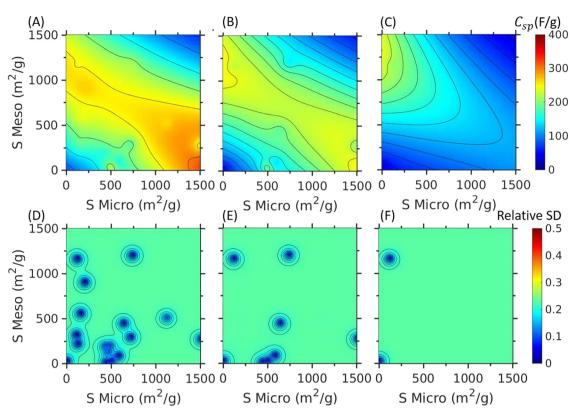
Fig. 5 Specific capacitance and relative standard deviation (standard deviation divided by the mean) *versus* the surface areas of micropores and mesopores predicted by PhysGPR with the rational quadratic kernel. (A)–(C) The predicted mean of the specific capacitance; (D)–(F) the relative standard deviation of the specific capacitance. The corresponding scan rates are (A), (D) 5 mV s<sup>-1</sup>, (B), (E) 50 mV s<sup>-1</sup>, and (C), (F) 200 mV s<sup>-1</sup>.
