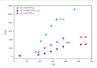
Fig. 4 TONs of different tris-WRCs 6c, 7a, and 9a. During long-term irradiation (700 mW Hg lamp), two equivalents of chromophore were added at every measurement point, until a total amount of 12 equiv., marked with a line
