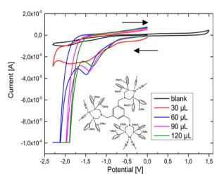
Fig. 2 Cyclic voltammogram of 8b at different water concentrations. Dry MeCN as solvent, electrodes: WE: glassy carbon GC, RE: Ag/AgNO<sub>3</sub>, CE: Pt (PF<sub>6</sub> is omitted for clarity in the figure).
