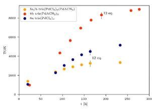
Fig. 3 TONs of palladium based tris-WRCs 8a-b. During the long-term irradiation (700 mW Hg lamp), two equivalents of chromophore were added at every measurement point, until a total amount of 12 equiv., marked with a line. The mixture of  $tris(PdCl_2)_2(PdACN_2)$  8a/b (yellow), in which the chloride was only partially substituted against ACN, displayed a lower TON of 3332 than the pure 8b with 8899
