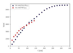
Fig. 6 TON comparison of  $tris(PdCl_2)_3$  **8a** (red) and  $tris(PdACN_2)_3$  **8b** (blue) with 12 equiv. of PS, 470 nm, 180 mW LED irradiation.
