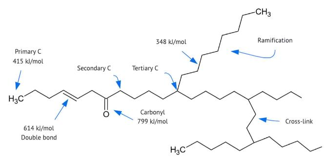
Fig. 3 Example section of a polyethylene macromolecule with possible deviations from the ideal structure and corresponding dissociation energy of some typical bonds. Values are related to the bonds made between carbon and carbon or hydrogen or oxygen. Source of values: Huheey, Keiter and Keiter, 1993.<sup>14</sup>
