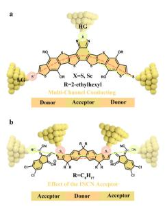
Fig. 4 (a) Multiple charge transfer pathways of donor-acceptor laddertype molecules. Reproduced with permission.<sup>31</sup> (b) Schematic illustration of single-molecule junctions for the acceptor-donor-acceptor structure using different anchor groups. Effect of the INCN acceptor on the electronic characteristics of the donor center after molecule protonation. Reproduced with permission.32
