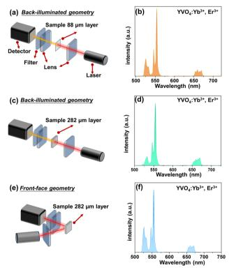
Fig. 2 (a, c and e) Schematic representation of the experimental setup, *i.e.* optical geometry for the UCL measurements and (b, d and f) the corresponding UC emission spectra for the YVO<sub>4</sub>:Yb<sup>3+</sup>, Er<sup>3+</sup> sample. (a–d) backilluminated excitation geometry for the 88  $\mu$ m thick sample (a and b), and for the 282  $\mu$ m thick sample (c and d); (e and f) front-face excitation geometry for the 282  $\mu$ m thick sample.
