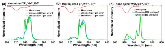
Fig. 3 Normalized UC emission spectra of (a) the nano-sized YVO<sub>4</sub>:Yb<sup>3+</sup>, Er<sup>3+</sup>, (b) micron-sized YF<sub>3</sub>:Yb<sup>3+</sup>, Er<sup>3+</sup>, and (c) nano-sized YF<sub>3</sub>:Yb<sup>3+</sup>, Er<sup>3+</sup>, recorded for different sample thicknesses; ( $\lambda_{ex}$ = 975 nm, bottom) combined with absorption spectra (top) of the obtained products.
