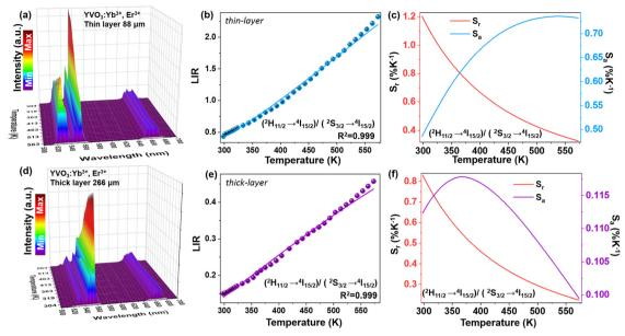
Fig. 5 (a and d) UC emission spectra of the thin-layer (a) and thick-layer (d) sample of YVO<sub>4</sub>: Er<sup>3+</sup>, Yb<sup>3+</sup> nanocrystals measured at increasing temperature values ( $\lambda_{\rm ex} = 975$  nm); (b and e) the determined LIR values (525/550 nm) and (c and f) the corresponding  $S_{\rm r}$  and  $S_{\rm a}$  values as a function of temperature, obtained for the thin-layer (b and c) and thick-layer (e and f) samples, respectively.
