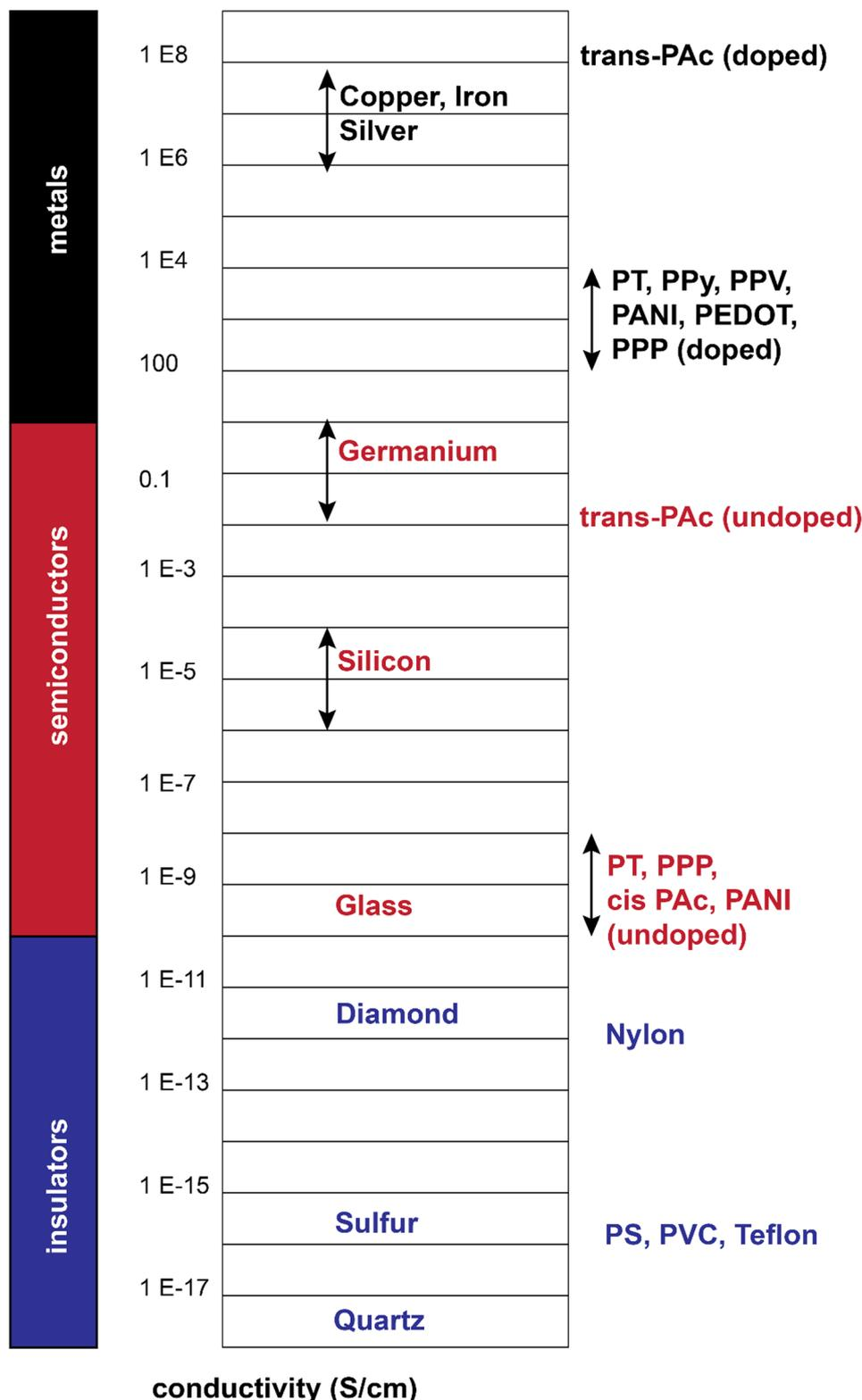
Fig. 4 Electrical conductivity of doped/undoped conjugated polymers relative to selective inorganic materials.<sup>22–24</sup>
