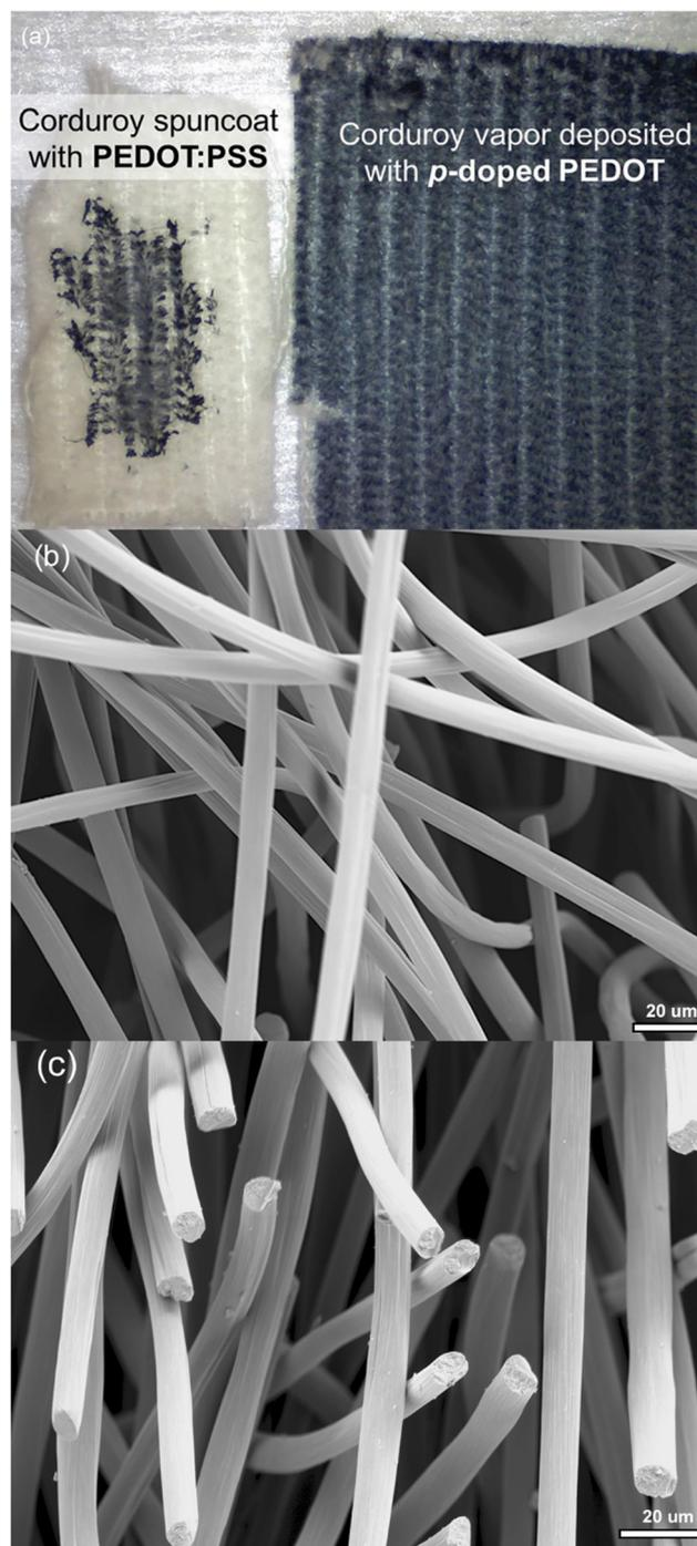
Fig. 8 (a) Corduroy swatch with 2 in<sup>2</sup> surface coated with PEDOT: PSS solution (left) and with 4 in<sup>2</sup> surface deposited with PEDOT via oCVD; reproduced from ref. 103 with permission from The Royal Society of Chemistry. (b) and (c) Microporous carbon felt uncoated and coated with PPy via oCVD, respectively.<sup>237</sup>
