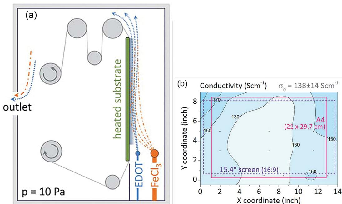
Fig. 9 (a) An illustration of the R2R oCVD reactor constructed in MIT; (b) PEDOT conductivity distribution deposited in an area of  $\sim 20 \text{ cm} \times 30 \text{ cm}$  at a deposition temperature of  $100 \text{ }^\circ\text{C}$ . Reproduced from ref. 272 with permission from The Royal Society of Chemistry.
