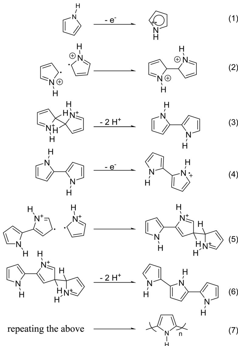
Scheme 1 Oxidation polymerization of PPy, based on the reaction mechanism proposed by Diaz *et al.*<sup>79</sup>
