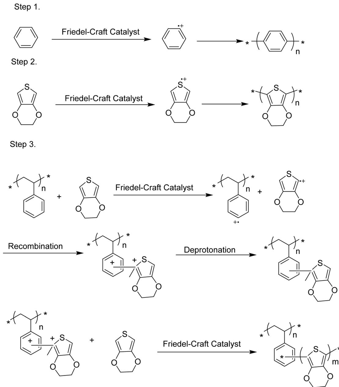
Scheme 3 The proposed mechanism of PEDOT grafting to a substrate having aromatic groups in its structure.<sup>255</sup>
