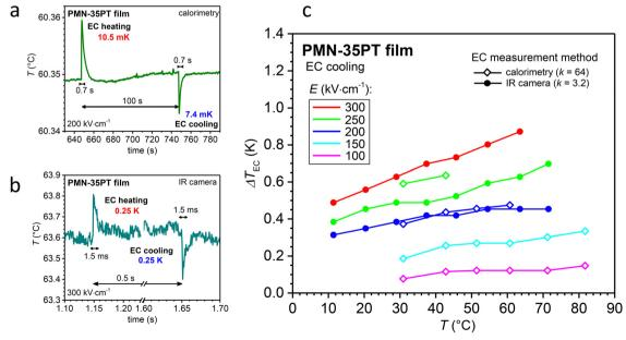
Fig. 5 Typical EC cycle obtained by (a) calorimeter method at 60.35 °C and 200 kV cm<sup>-1</sup> and (b) IR camera at 63.6 °C and 300 kV cm<sup>-1</sup>. (c) Temperature- and field-dependent  $\Delta T_{EC}$  values of the annealed PMN-35PT thick films measured by the calorimeter (open squares) and the IR camera (solid circles) methods
