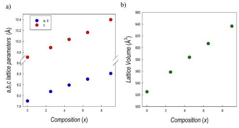
Fig. 8 Trend of (a) a = b and c lattice parameter, and (b) cell volume for the samples of the  $Cs_3Sb_2Br_{9-x}I_x$  solid solution as a function of x.
