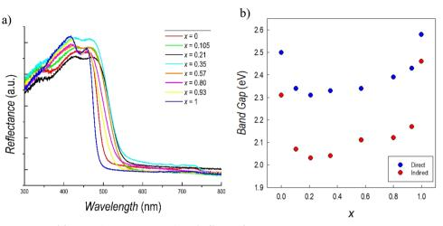
Fig. 5 (a) Reflectance spectra and (b) trend of the band gaps of the  $Cs_3(Sb_{1-x}Bi_x)_2Br_9$  solid solution
