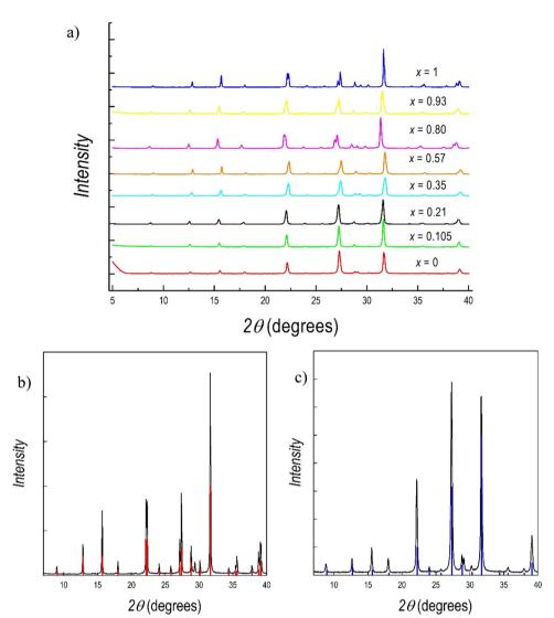
Fig. 2 (a) XRD patterns of a  $Cs_3(Sb_{1-x}Bi_x)_2Br_9$  solid solution as a function of x; (b) diffraction pattern of  $Cs_3Bi_2Br_9$  superimposed to the calculated pattern of the hexagonal structure (vertical red lines); and (c) diffraction pattern of  $Cs_3Sb_2Br_9$  superimposed to the calculated pattern of the hexagonal structure (vertical blue lines).
