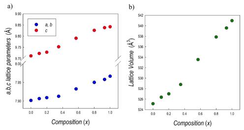
Trend of (a) a = b and c lattice parameters, (b) cell volume for the samples of the  $Cs_3(Sb_{1-x}Bi_x)_2Br_9$  solid solution as a function of x.
