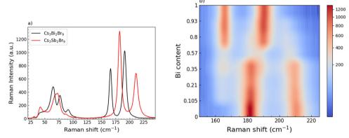
Fig. 4 (a) Comparison between room temperature (RT) Raman spectra of the end-members. (b) Color map reporting the modes intensity of the sample spectra in the range between 150 and 225  $\,\mathrm{cm}^{-1}$  as a function of Bi content (we applied a power-law normalization to remap the colors, to increase the contrast and better point out the change in the mode position).
