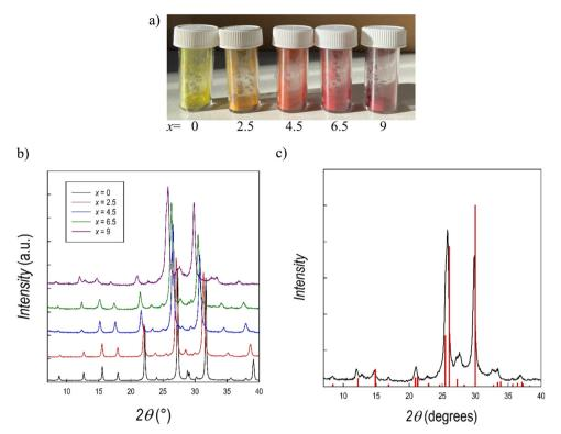
Fig. 7 (a) Photograph of the samples of  $Cs_3Sb_2Br_{9-x}I_x$  solid solution; (b) XRD patterns of the  $Cs_3Sb_2Br_{9-x}I_x$  solid solution, (c) XRD pattern of  $Cs_3Sb_2I_9$  against the calculated structure of the layered polymorph (e.g.  $P\overline{3}m1$ )
