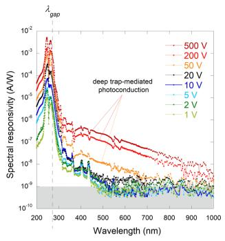
Fig. 7 Spectral responsivity of the  $\kappa$ -Ga<sub>2</sub>O<sub>3</sub> epitaxial thin film in the 200-1000 nm range at different bias voltages. Dashed line indicates the wavelength  $\lambda_{\text{gap}} \approx$  270 nm corresponding to the energy bandgap ( $\approx$ 4.6 eV). Measurement points within the grey band have to be considered below the background noise level.
