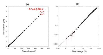
Fig. 2 Linear (a) and log-log (b) plots showing the current-voltage curves of the fabricated X-ray detector measured under dark conditions. Dashed line represents in both cases the best linear fit to the experimental data.
