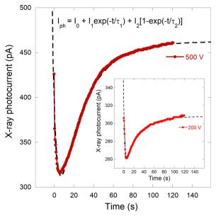
Fig. 6 Curve fitting to experimental data of X-ray photocurrent at  $V_{BIAS}$  = 500 V and (inset)  $V_{\rm BIAS}$  = 200 V. Dashed lines represent the best fit curves obtained by using eqn (1). For the sake of simplicity, the overshoot peaking time was assumed to be t = 0.
