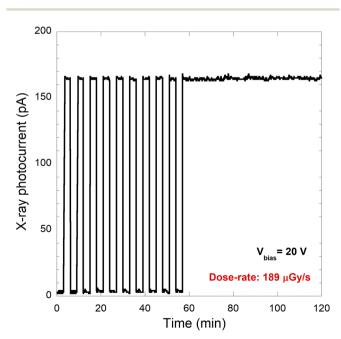
Fig. 9 X-ray photocurrent recorded with the fabricated  $\kappa$ -Ga<sub>2</sub>O<sub>3</sub>-based detector in a measurement session consisting of two parts: (1) 10 on-off cycles (6 min each); (2) 1 h of continuous irradiation. Bias voltage and dose rate were set to 20 V and 189  $\mu$ Gy s<sup>-1</sup>, respectively
