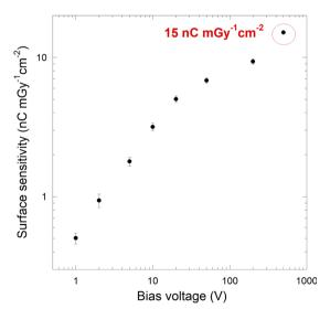
Fig. 5 Surface specific sensitivity of the fabricated X-ray κ-Ga<sub>2</sub>O<sub>3</sub> detector as a function of the bias voltage. Error bars are related to the linear fitting of the experimental data shown in Fig. 4(b).
