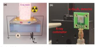
Fig. 1 (a) Operating scheme of the fabricated  $\kappa$ -Ga<sub>2</sub>O<sub>3</sub> photoconductive X-ray detector; (b) picture of the device mounted on a PCB board and positioned right in front of the X-ray collimator output slit.
