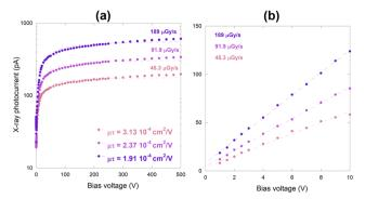
Fig. 10 (a) Experimental results for the evaluation of the average mobilitylifetime product at different dose rates. Bias voltage was varied in the 1-500 V range. In all the cases, dashed lines show the best fit to data obtained by using Hecht's eqn (2); (b) the same plot as Fig. 10(a) zoomed in the 1–10 V range, aimed at showing the ohmic behaviour of the metal contact under X-ray irradiation. Dashed lines represent the best linear fit to experimental data
