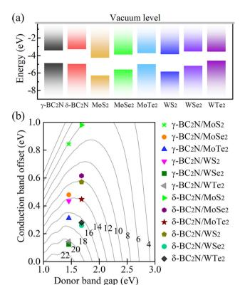
Fig. 11 (a) Band alignments and (b) PCE (in %).
