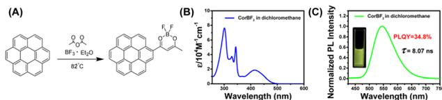
Fig. 2 (A) Cascade synthesis of luminescent  $\text{BF}_2\text{bdk}$  compounds. (B) UV-vis spectra of  $\text{CorBF}_2$  in the dichloromethane solution. (C) Steady-state emission spectra of  $\text{CorBF}_2$  in the dichloromethane solution.
