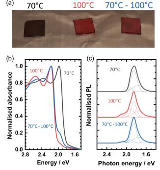
Fig. 3 (a) Optical image of OBESnI<sub>4</sub> thin films processed at 70 °C, 100 °C, and 70-100 °C. (b) Absorbance spectra and (c) photoluminescence spectra of the thin films.
