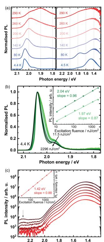
Fig. 2 (a) Temperature-dependent photoluminescence spectra of OBESnl<sub>4</sub> (left panel) and EDBESnI<sub>4</sub> (right panel). Power-dependent photoluminescence spectra at 4.4 K of (b) OBESnl<sub>4</sub> and (c) EDBESnl<sub>4</sub>, where the insets show the doublelogarithmic plots of the photoluminescence intensity versus excitation fluence.
