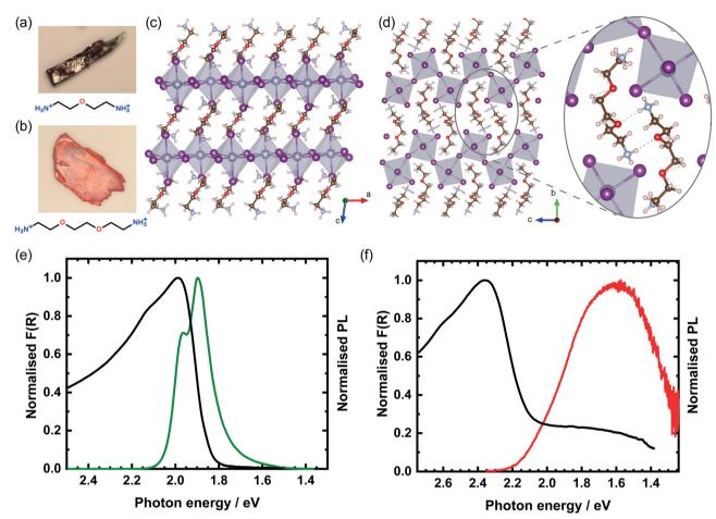
Fig. 1 (a) OBESnl<sub>4</sub> and (b) EDBESnl<sub>4</sub> images of mm-sized single crystals. Crystal structure of (c) OBESnl<sub>4</sub> and (d) EDBESnl<sub>4</sub>, where grey atoms are Sn, purple are I, blue are N, brown are C, red are O, and white are H. The inset highlights the formed hydrogen bonds. Kubelka–Munk transformed diffuse reflectance and photoluminescence spectra of (e) OBESnl<sub>4</sub> and (f) EDBESnl<sub>4</sub>.
