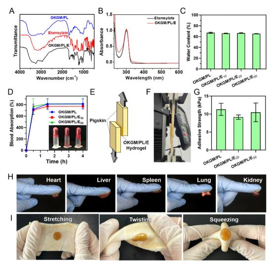
Fig. 3 (A) FTIR spectra, (B) UV spectra, (C) water content, and (D) blood absorption of the OKGM/PL/E hydrogels. (E) Schematic illustration and (F) photograph of the lap shear experiment. (G) Adhesive strength of the OKGM/PL/E hydrogels. (H) and (I) Photographs showing the adhesion property of the OKGM/PL/E<sub>50</sub> hydrogels.
