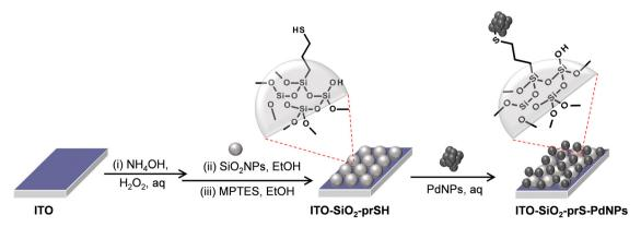
Scheme 1 Step-by-step fabrication of ITO-SiO<sub>2</sub>-prS-PdNPs as described in Section 2.5
