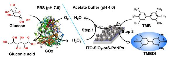
Scheme 3 Schematic representation of the colorimetric determination of glucose using ITO-SiO<sub>2</sub>-prS-PdNPs.
