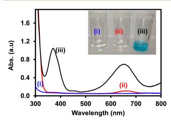
Fig. 2 UV-vis absorption spectra of (i) 0.20 M  $H_2O_2$  + ITO-SiO<sub>2</sub>-prS-PdNPs, (ii) 4.2 mM TMB + ITO-SiO $_2$ -prS-PdNPs and (iii) 0.20 M H $_2$ O $_2$  + 4.2 mM TMB + ITO-SiO<sub>2</sub>-prS-PdNPs (The inset photograph for the corresponding colour change of different reaction systems). All were measured in 0.20 M acetate buffer (pH 4.0).
