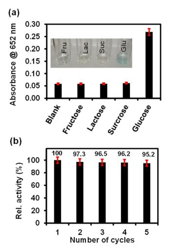
Fig. 6 (a) Selectivity of the colorimetric assay for glucose detection and other interfering substances for ITO-SiO2-prS-PdNPs (inset: The corresponding images of the reaction solutions) and (b) reusability of ITO-SiO<sub>2</sub>prS-PdNPs towards the detection of glucose.
