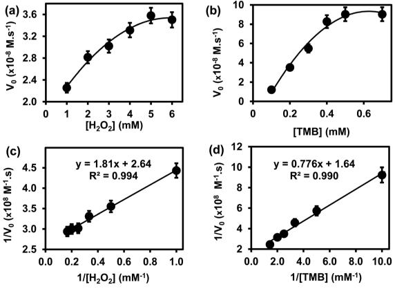
Fig. 4 The steady-state kinetic plots of the ITO-SiO<sub>2</sub>-prS-PdNPs (a) varying  $[H_2O_2]$  at a fixed [TMB], (b) varying [TMB] at a fixed  $[H_2O_2]$  and their corresponding double reciprocal plots (c)  $[H_2O_2]$  at a fixed [TMB] and (d) [TMB] at a fixed  $[H_2O_2]$
