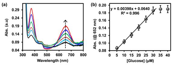
Fig. 5 (a) UV-vis absorption spectra and (b) the corresponding linear calibration curve of glucose detection using ITO-SiO<sub>2</sub>-prS-PdNPs
