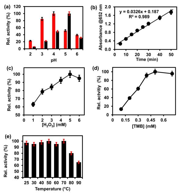
Fig. 3 Effect of (a) pH (red), (b) reaction time and changing concentrations of (c)  $H_2O_2$  and (d) TMB, and (e) temperature on the peroxidase-like activity of ITO-SiO<sub>2</sub>-prS-PdNPs. (Effect of pH (a) (black) on the peroxidase-like activity of PdNPs).
