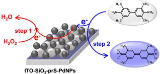
Scheme 2 ITO-SiO<sub>2</sub>-prS-PdNP electron-transfer mechanism for TMB oxidation in 10 mM acetate buffer (pH 4.0).
