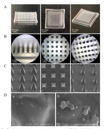
Fig. 5 Morphological characterization images of DMNs. (A) € direct view of the DMNs taken by the camera; (B) the shape of the DMN tips under an optical microscope; (C) the SEM images of DMNs; and (D) images of the dispersion of ZnO NPs in DMNs by SEM (a, DMNs based on ZnO NPs/IL; b, DMNs based on ZnO NPs/DIW).
