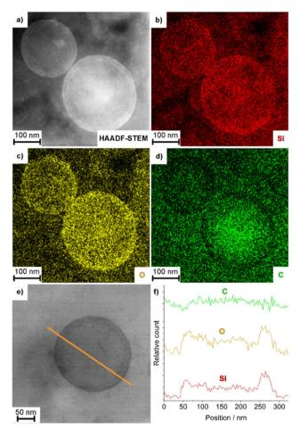
Fig. 3 Nanostructure of AMC@SiO $_2$  core@shell nanocarriers: (a) HAADF-TEM image, (b-d) EDXS area scans (Si-K, O-K, C-K lines used for analysis) of the nanostructure shown in (a), (e and f) EDXS line scan with (f) element mapping along the orange line in (e).
