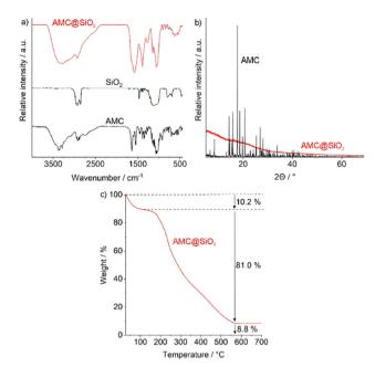
Fig. 4 Chemical composition of the as-prepared AMC@SiO2 core@shell nanocarriers: (a) FT-IR spectrum with pure AMC and SiO<sub>2</sub> as references, (b) XRD with AMC as a reference, (c) TG analysis
