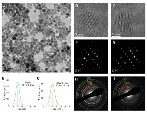
Fig. 1 (A) TEM image of Zn<sub>0.4</sub>Fe<sub>2.6</sub>O<sub>4</sub> NPs prepared under high temperature with autogenous pressure; (B) and (C) size distributions; (D) and (E) HRTEM images; (F) and (G) FFT patterns down the [211] axis; and (H) and (I) selected area electron diffraction (SAED) patterns with denoted crystal planes for iron oxide and Zn<sub>0.4</sub>Fe<sub>2.6</sub>O<sub>4</sub> NPs respectively
