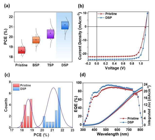
Fig. 5 (a) Statistical analysis of PCE for pristine, BSP, TSP and DSP devices. (b) J-V characteristics of pristine and DSP based devices. (c) Statistical histogram of PCE for pristine and DSP devices. (d) External quantum efficiency curves of the pristine and DSP based devices.
