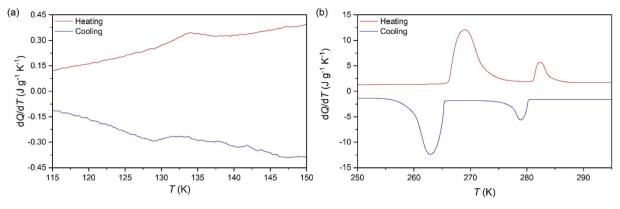
Fig. 1 VT-DSC curves for the [DBA][BF<sub>4</sub>] compound in the (a) lower- and (b) higher-temperature ranges.
