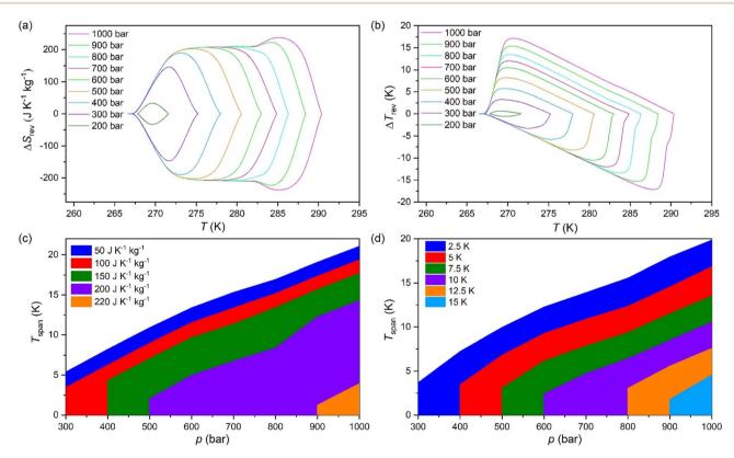
Fig. 4 (a) Pressure-driven reversible isothermal entropy changes on applying  $(0 \to p)$  and removing  $(p \to 0)$  pressure. (b) Reversible adiabatic temperature changes on applying  $(0 \to p)$  and removing  $(p \to 0)$  pressure at different pressures. (c) Temperature span as a function of applied pressure for fixed intervals of reversible isothermal entropy changes and (d) reversible adiabatic temperature changes for [DBA][BF<sub>4</sub>].
