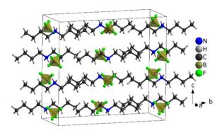
Fig. 7 Structure of [DBA][BF $_4$ ] at 100 K (PIV), where the tetrahedra correspond to [BF $_4$ ] $^-$  anions and the chains to [DBA] $^+$  cations and the black cage represents the unit cell.
