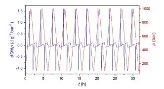
Fig. 5 Heat flow on pressurization/depressurization cycles over time
