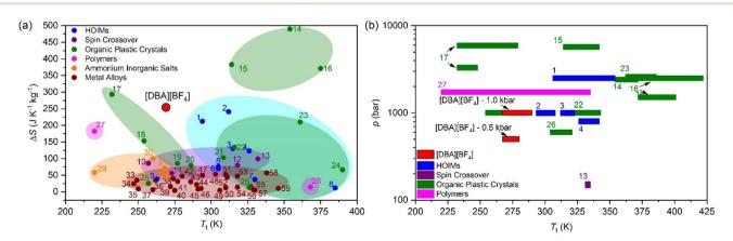
Fig. 6 (a) All barocaloric material temperature transition ( $T_t$ ) and entropy change ( $\Delta S$ ) comparison. (b) Operating temperature range and the needed pressure of the largest entropy change materials (>100 J K<sup>-1</sup> kg<sup>-1</sup>). See more information of all materials represented in Table S2 of the ESI†.
