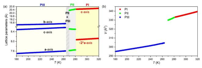
Fig. 11 Evolution of (a) the lattice parameters and (b) the volume of PI, PII and PIII of [DBA][BF<sub>4</sub>] as a function of temperature. Note: blue, green and red points represent the lattice parameters and volume of the polymorphs PIII, PII an PI, respectively. Note: error bars, as calculated by using the software, are smaller than symbols.
