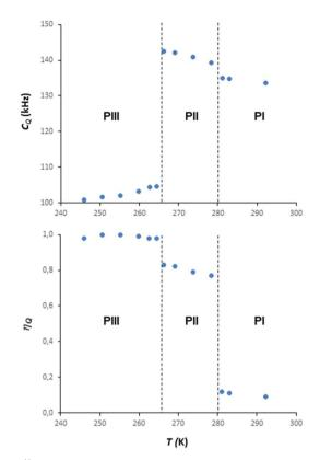
Fig. 14 <sup>11</sup>B quadrupolar parameters as a function of sample temperature (on heating).
