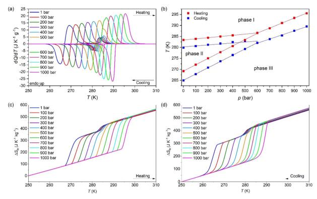
Fig. 3 (a) VP-DSC curves of [DBA][BF4] under isobaric conditions from 1 bar to 1000 bar. (b) Temperature of the maximum of each peak of the VP-DSC curves on cooling and heating as a function of the applied pressure. (c)  $\Delta S_{ib}$  curves at different pressures during heating and (d) cooling.
