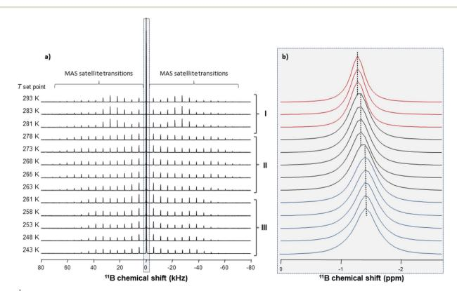
Fig. 13  $^{1}$ B MAS NMR spectra obtained at different temperatures ( $\nu_{0} = 193$  MHz and  $\nu_{MAS} = 5.5$  kHz): (a) full spectral window showing the MAS satellite transition sidebands; (b) zoomed-in view of the isotropic centre band.
