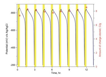
Fig. 6 F-PCN cyclability (multiple time 20 minute photo-charging and subsequently electrical discharging with a current density of 2 mA  $\rm g^{-1}$ ) using 0.1 M  $\rm K_2SO_4$  and 5 mM 4-MBA electrolyte.
