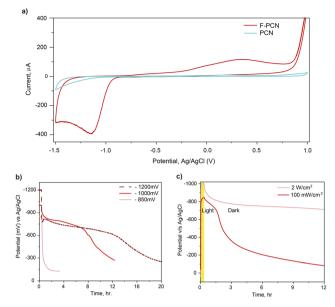
Fig. 2 (a) Cyclic voltammetry curve for PCN and F-PCN in 0.1 M Na<sub>2</sub>SO<sub>4</sub> and 5 mM 4-MBA, scan rate 5 mV s<sup>-1</sup> (b) charging F-PCN for 20 min with three different external biases in Na<sub>2</sub>SO<sub>4</sub> and 4-MBA electrolyte (c) charging F-PCN in Na<sub>2</sub>SO<sub>4</sub> and 4-MBA with different intensity lamp (1.5 AM). All the measurements are done under inert conditions
