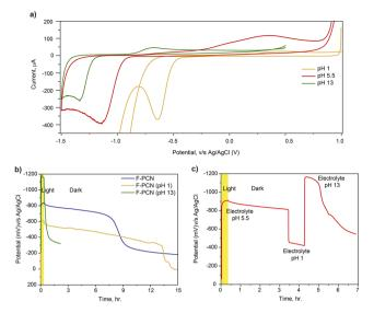
Fig. 5 (a) Cyclic voltammetry on F-PCN at different pH of the electrolyte (M<sub>2</sub>SO<sub>4</sub> and 4-MBA) (b) OCP measurement of F-PCN at different pH of the electrolyte (M2SO4 and 4-MBA) (c) OCP measurement on F-PCN, pH of electrolyte changed from 5.5 to 1 after 3 h of dark and again the pH to 13 after 4 h of dark.
