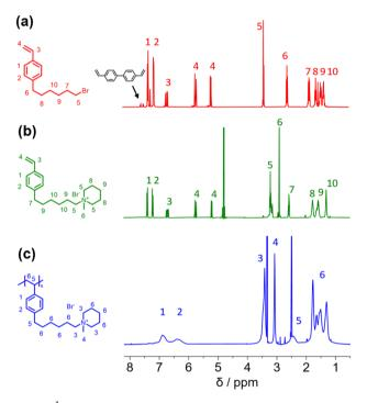
Fig. 2 (a) <sup>1</sup>H NMR spectra of 4-(6-bromohexyl)styrene (b) 1-methyl-(6-(4-vinylphenyl)hexyl)piperidin-1-ium bromide (c) poly(1-methyl-(6-(4-vinylphenyl)hexyl)piperidin-1-ium bromide).
