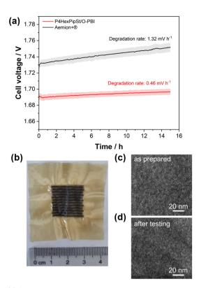
Fig. 7 (a) Cell voltage during the constant current hold at 1 A cm<sup>-2</sup> for the blend membrane and Aemion+®, whereby the shaded area represents one standard deviation from the mean value of three independent measurements. (b) Blend membrane after the constant current hold with catalyst residues on the membrane. (c) HAADF-STEM image of the membrane before testing. (d) HAADF-STEM image of the membrane after the constant current hold.
