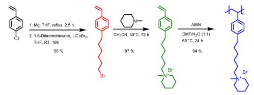
Fig. 1 Synthesis of poly(1-methyl-(6-(4-vinylphenyl))piperidin-1-ium bromide): (1) coupling of 1,6-dibromohexane to a styryl Grignard. (2) Quaternization with *N*-methylpiperidine. (3) Free radical polymerization to yield P4HexPipSt.
