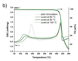
Fig. 3 (a) IR spectra of the plain formulation (grey) and the sample cured at 90 °C (green). (b) STA of the plain formulation (grey) and the photo-DSC cured samples at 80 °C (green solid), 90 °C (black solid) and 100 °C (green dot)
