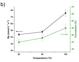
Fig. 2 (a) Photo-DSC of the PT-30 formulation at 80-100 °C,  $2 \times 900$  s, 320-500 nm, 60 mW cm<sup>-2</sup>. (b) Temperature dependence of rate of polymerization (R<sub>p</sub> black) and conversion of the cyanate ester groups (green).
