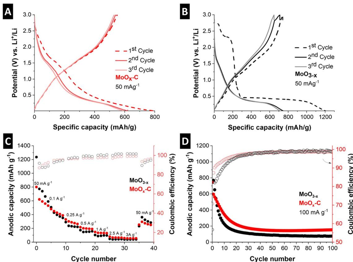
Fig. 7 (A) Galvanostatic charge–discharge curves of MoO<sub>x</sub>-C and (B) MoO<sub>3-x</sub> at a specific current of 50 mA g<sup>-1</sup> in the potential range of 0.01 V to 3 V vs. Li<sup>+</sup>/Li, (C) rate performance of MoO<sub>3-x</sub> and MoO<sub>x</sub>-C at rates from 50 mA g<sup>-1</sup> to 3 A g<sup>-1</sup>, (D) stability test of MoO<sub>3-x</sub> and MoO<sub>x</sub>-C cycled at 100 mA g<sup>-1</sup>.
