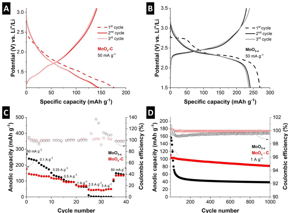
Fig. 6 First three galvanostatic charge–discharge cycles of (A) MoO<sub>x</sub>-C and (B) MoO<sub>3-x</sub> at 50 mA g<sup>-1</sup>, (C) rate capability tests at various specific current values from 50 mA g<sup>-1</sup> to 3 A g<sup>-1</sup>, then back to 50 mA g<sup>-1</sup>, in the voltage range 1.5 V to 3.5 V for MoO<sub>3-x</sub> and 1.1 V to 3.1 V for MoO<sub>x</sub>-C, (D) cycling stability test for MoO<sub>3-x</sub> and MoO<sub>x</sub>-C at 1 A g<sup>-1</sup> for 1000 cycles.
