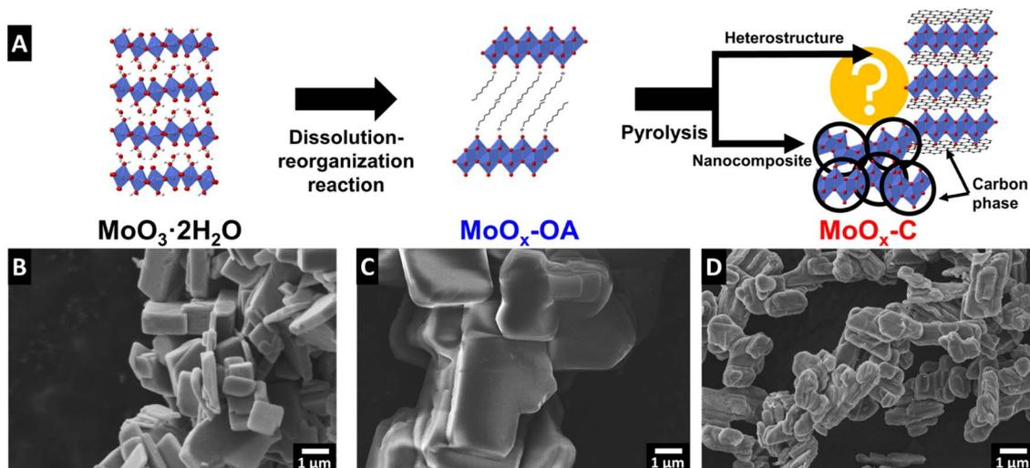
Fig. 1 (A) Schematic illustration of the synthesis process: octylamine is assembled in the  $\text{MoO}_3 \cdot 2\text{H}_2\text{O}$  interlayer space via a dissolution–reorganization reaction; subsequent pyrolysis yields the carbon-containing nanocomposite. SEM images of (B) molybdenum oxide dihydrate ( $\text{MoO}_3 \cdot 2\text{H}_2\text{O}$ ), (C)  $\text{MoO}_x\text{-OA}$ , and (D)  $\text{MoO}_x\text{-C}$  after pyrolysis in argon at  $700^\circ\text{C}$ .
