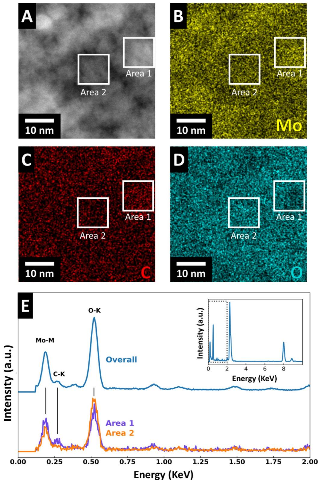
Fig. 5 (A) HAADF-STEM micrograph showing Z-number contrast and (B–D) EDS mapping with elemental distribution of Mo, C, and O in  $\text{MoO}_x$ –C. (E) Chemical analysis of the two marked areas by quantitative STEM-EDS spectral imaging analysis.
