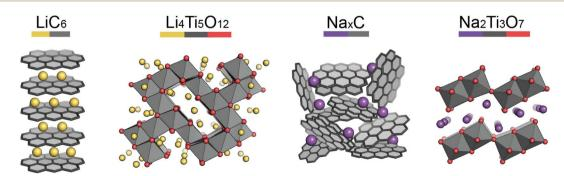
Fig. 3 Structures of the key anode materials covered in this review. (Left to right) Graphite, lithium titanate, hard carbon, sodium titanate. Element colours are shown by the coloured bar under the formulae.
