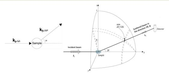
Fig. 5 (Left) Vector representation of a particle scattered by a sample. (Right) Geometry for a scattering experiment. Reproduced with permission from ref. 20. Copyright 2016, Elsevier Ltd.
