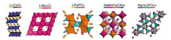
Fig. 2 Structures of the key cathode materials covered in this review. Left to right: layered oxide (which NMC, NCA, and the Na-ion P2 and O3 materials are based on), LMO, LFP, PBA, NASICON. Element colours are shown by the coloured bar under the formulae.
