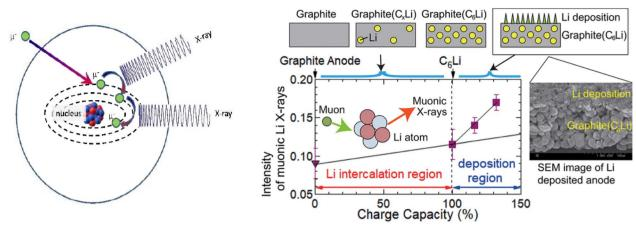
Fig. 29 (Left) Schematic representation of the muon capture and travel through the electron shells of an atom. Reproduced with permission from ref. 145. Copyright © 2022, by the authors according to MDPI's open access policy. (Right) Intensity of muonic X-rays from metallic lithium growth in a graphite anode as a function of overcharge. Reproduced with permission from ref. 146. Copyright © 2020 American Chemical Society.
