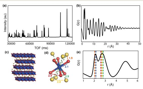
Fig. 10 Calculated neutron scattering (a) and PDF (b) of LiCoO<sub>2</sub>, the layered structure is shown in (c) and the CoO<sub>6</sub> sub-unit is shown in (d), with interatomic distances represented by dashed lines, and the corresponding positions in the PDF shown in the low-r region (e). The Co, O, and Li are represented by blue, red, and yellow spheres, respectively.
