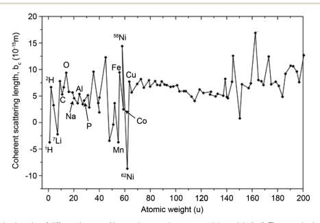
Fig. 6 Neutron scattering lengths of different isotopes (those relevant to battery materials are labelled). The magnitude of b is indicative of the isotope's scattering strength and its sign indicates a 180° phase difference relative to values with the opposite sign.
