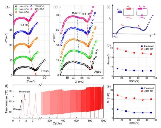
Fig. 2 EIS spectra at different SOCs for a (a) fresh cell and (b) an aged cell; (c) schematic illustration and an equivalent circuit used to fit the EIS Nyquist plots; the fitted results for (d)  $R_{\text{sei}}$ , and (e)  $R_{\text{ct}}$ ; (f) the temperature tested using a temperature sensing probe on the outer surface of the cell.
