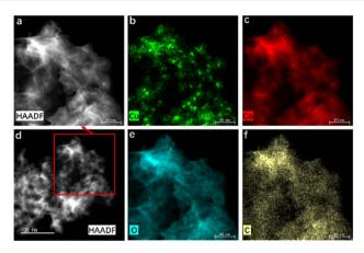
Fig. 3 (a and d) HAADF-STEM images of  $Cu@CoO_x$  derived from Cu-Co-MOF-74 and the corresponding elemental mapping images of (b) Cu, (c) Co, (e) O and (f) C.
