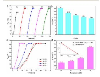
Fig. 1 (a and b) Durability of catalytic AB hydrolysis over 5 cycles at 25° C, and (c and d) temperature dependence of gas evolution of AB hydrolysis and the corresponding TOF values over Cu-Co-MOF-74 (inset in (d) is the Arrhenius plot (ln TOF) vs. 1/T) ( $n_{Co} = 0.204$  mmol,  $n_{\text{Cu}} = 0.005 \text{ mmol}, n_{\text{AB}} = 1 \text{ mmol}.$
