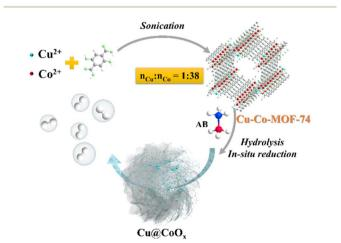
Scheme 1 Schematic illustration of the synthesis of Cu@CoO<sub>x</sub> from Cu-Co-MOF-74.
