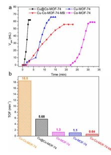
Fig. 4 (a) Gas evolution from aqueous AB and (b) the corresponding TOF values using control samples (25 °C, initial weight of MOF is 50 mg,  $n_{\rm AB}=1$  mmol).
