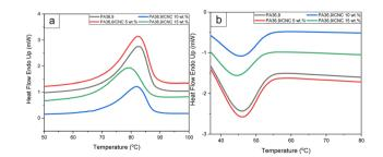
Fig. 3 DSC thermograms of PA36,9 (ref. 9) and PA36,9/CNC nano-composites with different CNC contents: (a) heating and (b) cooling.
