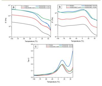
Fig. 5 DMA curves of PA36,9 and PA36,9/CNC nanocomposites with different CNC contents, as a function of temperature: the (a) storage modulus (E'), (b) loss modulus (E''), and (c) loss factor (tan  $\delta$ ).
