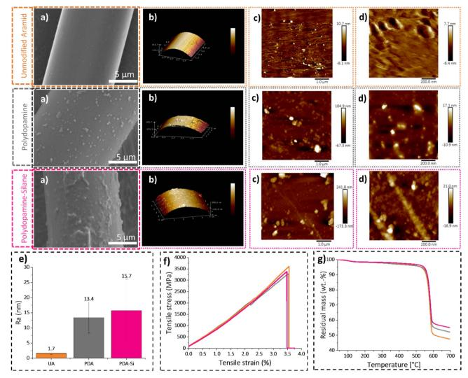
(a) SEM images of the fiber surface, (b) AFM 3D view of the fiber surface with a scan size of  $5 \mu m \times 5 \mu m$ , (c) 2D view of the fiber topography with a scan size of  $5 \mu m \times 5 \mu m$ , (d) 2D view of the fiber topography with a scan size of  $1 \mu m \times 1 \mu m$ , and (e) calculated roughness parameters. (f) Mechanical properties and (g) thermogravimetric analysis of UA (orange), PDA (grey) and PDA Si (pink).
