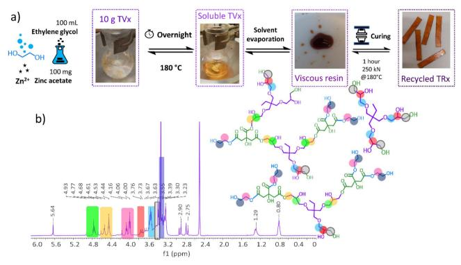
Fig. 7 (a) Chemical recycling methodology through transesterification exchange reactions. (b) Spectroscopic characterization of the viscous resin performed in deuterated DMSO by <sup>1</sup>H NMR.
