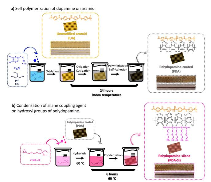
Fig. 1 The experimental setup followed to functionalize unmodified aramid fibers and meshes in two steps. (a) Self polymerization of dopamine. (b) Condensation of a silane coupling agent.
