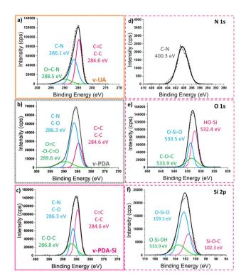
Fig. 3 XPS analysis. C 1s high resolution spectra of (a) virgin unmodified aramid (v-UA), (b) virgin polydopamine coated aramid (v-PDA), and (c) virgin polydopamine-silane functionalized aramid (v-PDA-Si). (d) N 1s, (e) O 1s and (f) Si 2p high resolution spectra of v-PDA-Si. The images include the analysis of deconvoluted curves and functional groups assigned to the fitted peaks. Dashed black lines correspond to the experimental curve. Solid black lines correspond to the fitted envelop.
