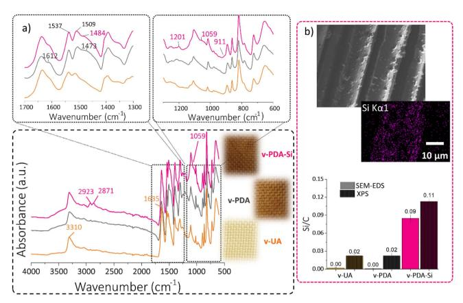
Fig. 2 Spectroscopic characterization of virgin aramid meshes of unmodified aramid (v-UA), polydopamine coated (PDA) and polydopamine silane functionalized (PDA-Si). (a) Acquired ATR FTIR spectra. (b) SEM-EDS mapping image of PDA-Si meshes and Si/C ratios determined by means of EDS and XPS measurements on the virgin meshes.
