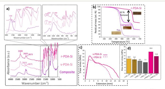
Fig. 10 (a) Spectroscopic characterization of recovered r-PDA-Si depicting the removal of the thermoset matrix supported by (b) thermogravimetric analysis indicating a removal of 82% of the thermoset matrix. (c) Typical lap-shear test curves comparing the performance of v-PDA-Si and r-PDA-Si after chemical recycling. (d) Comparison of the maximum shear stress obtained with UA, PDA and PDA-Si meshes in their virgin state and after chemical recycling
