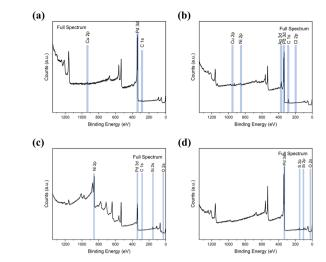
Fig. 3 XPS full survey spectra of waste metal wires (a), peeled flakes (b), e-beam evaporated electrodes from recycled Pd (c) and commercial Pd (d) on SiO<sub>2</sub>.
