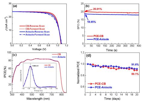
Fig. 6 (a) The J-V curves of the best PSCs prepared from spiro-OMeTAD films processed using different solvents. (b) The steady output of the best PSCs, (c) the IPCE spectra, and (d) the stability of PSCs.
