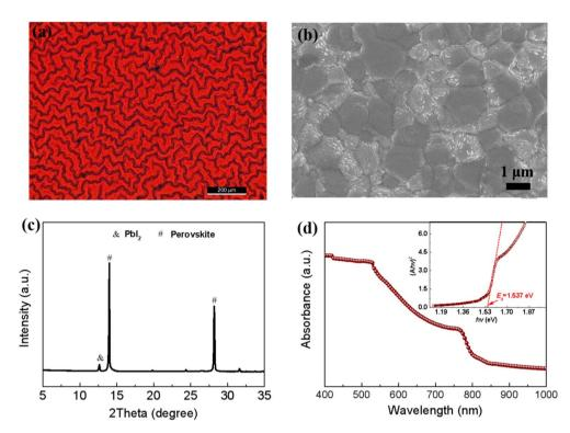
Fig. 3 The characterization of the perovskite films prepared by green solvent engineering. (a) An optical microscopy image, (b) the surface SEM image, (c) the XRD curves, and (d) the UV-Vis absorption spectra, where the inset shows the bandgap  $(E_g)$  fitting based on the relationship between  $(Ahv)^2 - hv$ .
