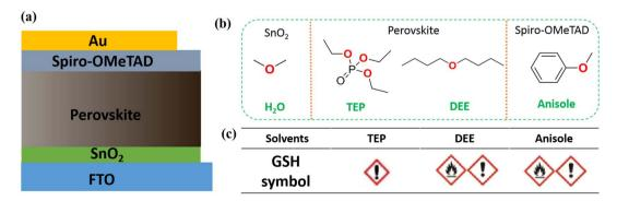
Fig. 1 (a) The device structure of typical efficient PSCs. (b) The molecular structure of solvents used for the preparation of various functional layers in the PSCs. (c) The GHS symbols of the solvents.
