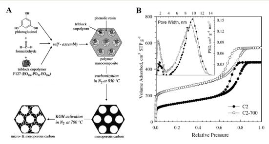
Fig. 3 (A) A common soft-templating system to prepare highly ordered mesoporous carbons, and then micropores on their wall via KOH activation. (B)  $N_2$  adsorption—desorption isotherms before (C2) and after the KOH activation step (C2-700) (inset shows the pore size distribution derived from these isotherms). Reproduced from ref. 32 with slight modification. Copyright 2008 Elsevier.
