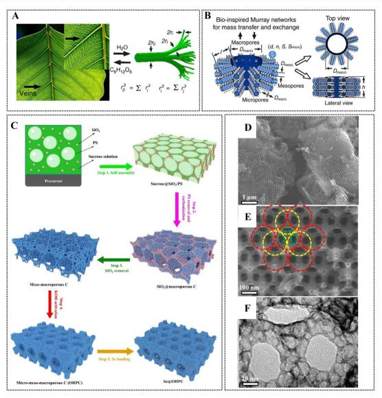
Fig. 2 (A and B) Hierarchically designed pore network to achieve efficient mass transfer following Murray's law.<sup>26</sup> (C) A method to prepare hierarchically porous Se-doped carbon as cathode for Li-Se batteries. (D and E) SEM and (F) TEM images of the prepared hierarchically porous material. Reproduced from ref. 23. Copyright 2022 Elsevier.
