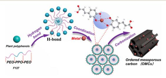
Fig. 8 Schematic representation of the metal-ion assisted coordination-induced self-assembly approach yielding metal-doped ordered mesoporous carbons using plant-derived polyphenols. Reproduced from ref. 75 with some modifications. In the upper part caffeic acid is depicted as it coordinates with a metal ion. Copyright 2023 Elsevier.
