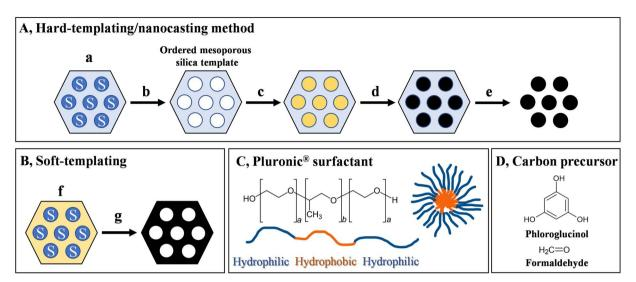
Fig. 5 (A) Hard- vs. (B) soft-templating methods. (C) Pluronic® surfactant and (D) the phloroglucinol–formaldehyde resin as structure directing agent and carbon precursor, respectively, for typical soft-templating methods.
