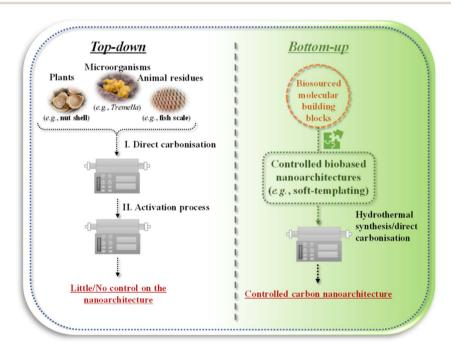
Different concepts of fabricating biobased nanoporous carbons through (left) "top-down" or (right) "bottom-up" strategies.
