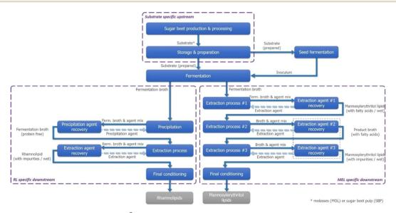
Fig. 1 Simplified aggregated flow diagram of Bio<sup>2</sup>-processes for the production of rhamnolipids (RL) and mannosylerythritol lipids (MEL); process stages represent different pooled process modules; recycling flows lead back to modules of use by the dotted line.
