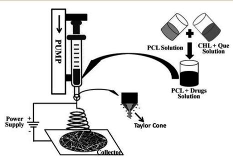
Fig. 12 Fabrication of a poly(caprolactone)-based nanofiber membrane functionalized with CHL and quercetin. 155
