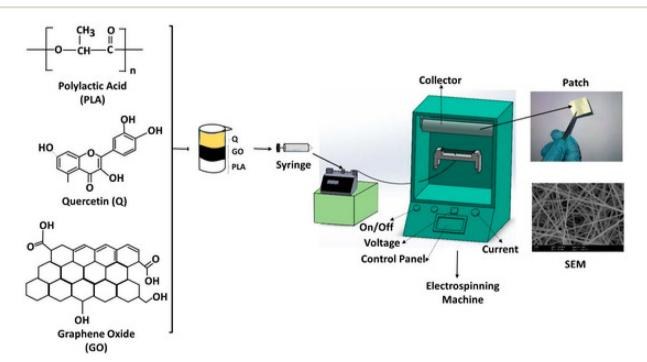
Fig. 11 Fabrication of PLA/GO/Q by electrospinning.92
