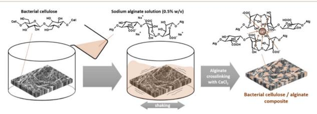
Fig. 8 Fabrication of bacterial cellulose/alginate composite. 130
