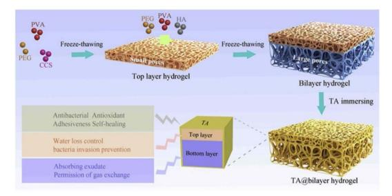
Fig. 7 Preparation process of TA@bilayer hydrogel.85
