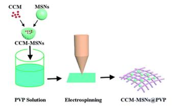
Fig. 4 Fabrication of curcumin-loaded mesoporous silica nanofiber mats.114
