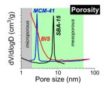
Fig. 2 A comparison of the XRD and pore size distribution of bioinspired silica with two archetypal ordered mesoporous silica materials, SBA-15 and MCM-41. Part of this figure is reproduced with permission from ACS Publications.<sup>28</sup>
